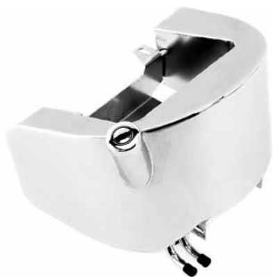
K90034 WINGED OIL TANK / 180/200/230-250 TIRE FRAMES 3 QT SIDE FILL / CHROME
