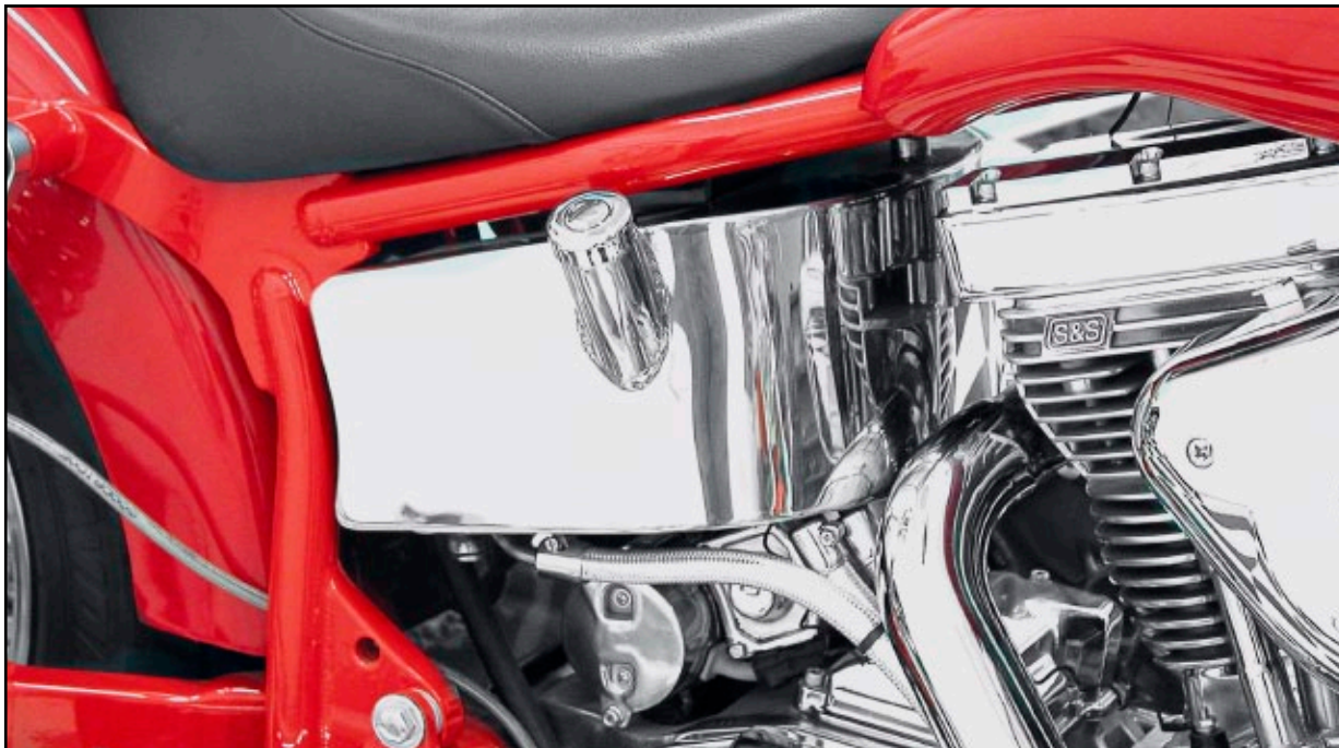
K90109 OIL TANK/WINGED HORSESHOE . . . POLISHED STAINLESS / 4 QT SIDE FILL / FOR STOCK & 180/200 FXR-STYLE FRAMES
